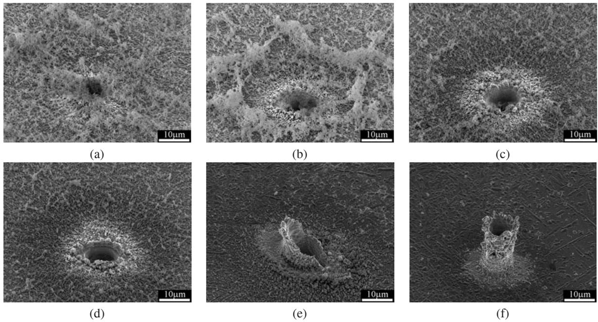
Figure 10: SEM images taken from the entrance of laser holes drilled in air using a rotating polarization, an energy of  $6.8 \mu\text{J}$  and 30000 pulses per hole. The pulse lengths presented here are (a) 150 fs, (b) 1 ps, (c) 10 ps, (d) 35 ps, (e) 220 ps and (f) 7 ns.
