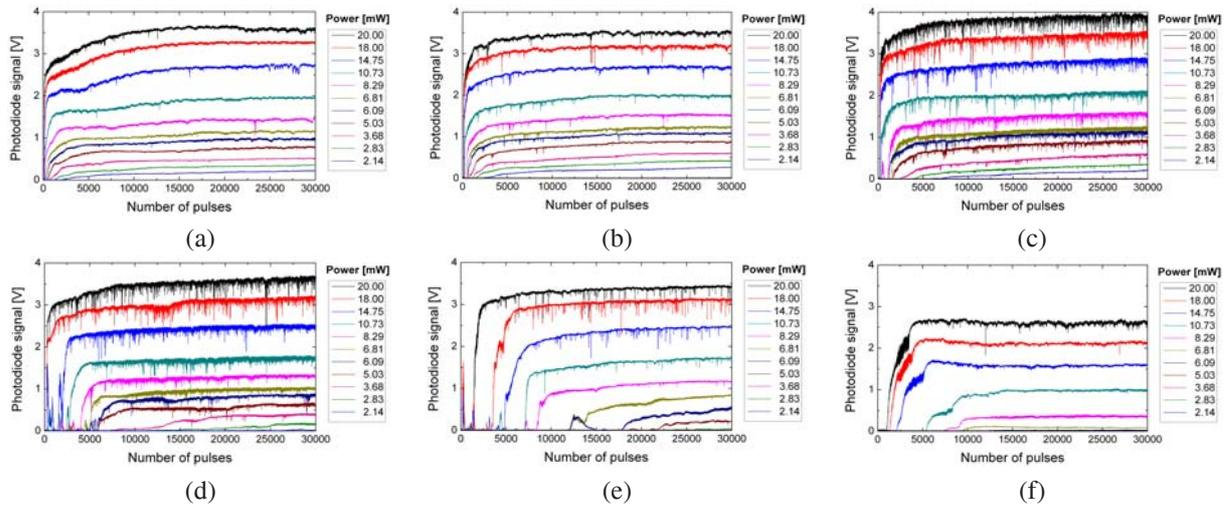
Figure 5: Photodiode results for holes drilled in air using 30000 pulses per hole. The pulse lengths presented here are (a) 150 fs, (b) 1 ps, (c) 10 ps, (d) 35 ps, (e) 220 ps and (f) 7 ns.
