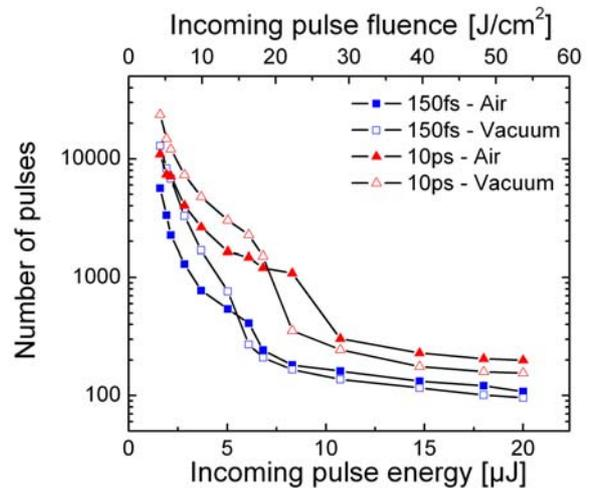
Figure 14: Number of pulses to go through a  $100 \mu\text{m}$  thick copper sheet as a function of laser pulse energy for two pulse lengths in air and vacuum.
