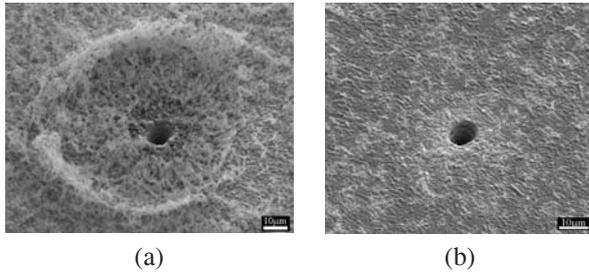
Figure 12: SEM micrograph of the entrance of a laser hole drilled with a pulse length of 150 fs, an energy of  $0.89 \mu\text{J}$  and 1000 pulses (a) in air and (b) in vacuum.
