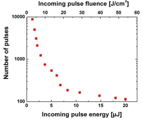
Figure 3: Number of pulses to go through the 100  $\mu\text{m}$  thick copper sheet at 150 fs in air.
