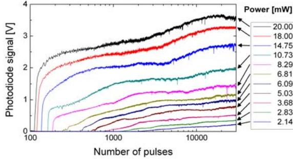
Figure 2: Results from the photodiode under the sample while drilling holes at 150 fs in air with various pulse energies.
