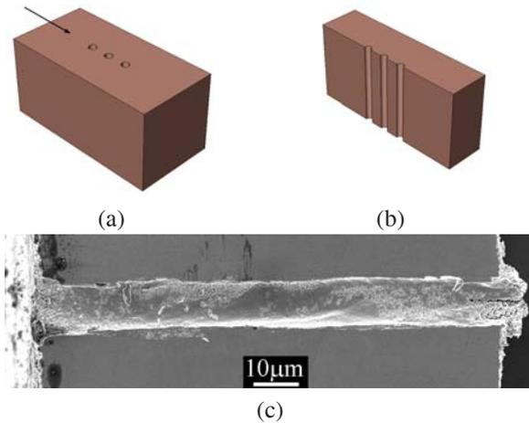
Figure 1: Schematic drawing showing (a) a  $100\ \mu\text{m}$  thick sheet containing  $10\ \mu\text{m}$  diameter through holes and (b) the results of a microtome cut. (c) Cross section of a laser hole drilled in air with 30000 pulses per holes and with a pulse length of 35 ps.
