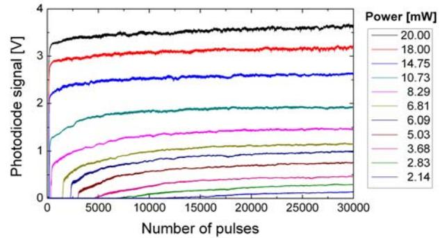
Figure 13: Signal from the photodiode while drilling in vacuum with 10 ps pulses.
