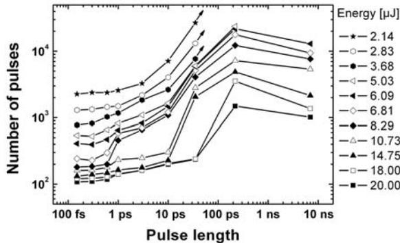
Figure 7: Number of pulses needed to go through a  $100\mu\text{m}$  thick copper sheet as a function of the pulse length for different pulse energies in air.
