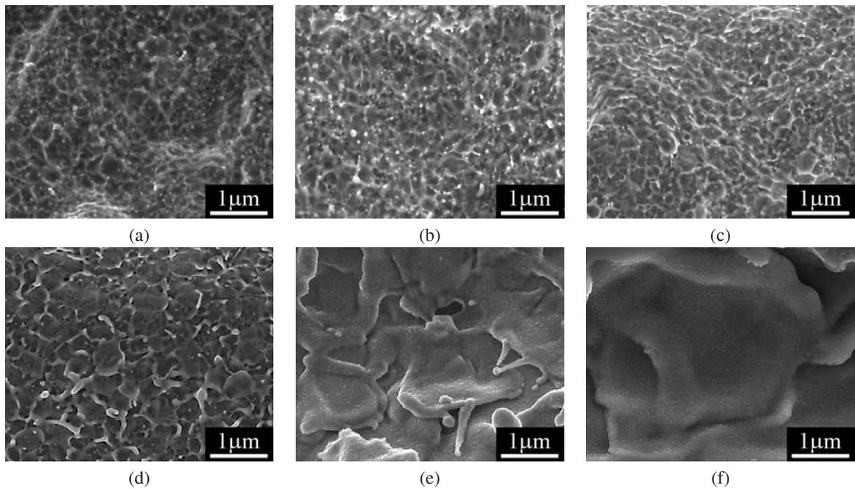
Figure 9: SEM images taken from the middle of laser-produced holes drilled in vacuum using a rotating laser polarization, an energy of  $10 \mu\text{J}$  and 30000 pulses per hole. The pulse lengths presented here are (a) 150 fs, (b) 1 ps, (c) 10 ps, (d) 35 ps, (e) 220 ps and (f) 7 ns.
