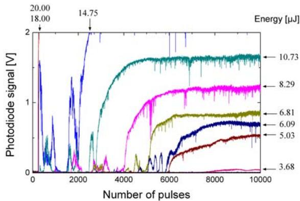
Figure 6: Close-up of figure 5(d) showing spikes in the early stages of drilling.
