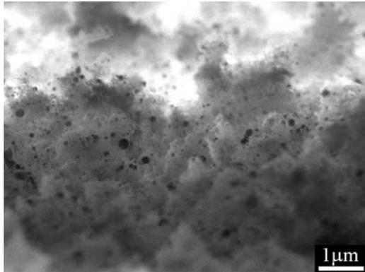
Figure 11: SEM image of the debris deposited close to a 10 ps laser hole drilled in air showing the small copper particles trapped in a much finer nanostructured foam.
