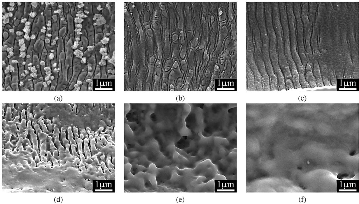
Figure 8: SEM images taken from the middle of laser-produced holes drilled in air using a rotating laser polarization, an energy of  $10 \mu\text{J}$  and 30000 pulses per hole. The pulse lengths presented here are (a) 150 fs, (b) 1 ps, (c) 10 ps, (d) 35 ps, (e) 220 ps and (f) 7 ns.
