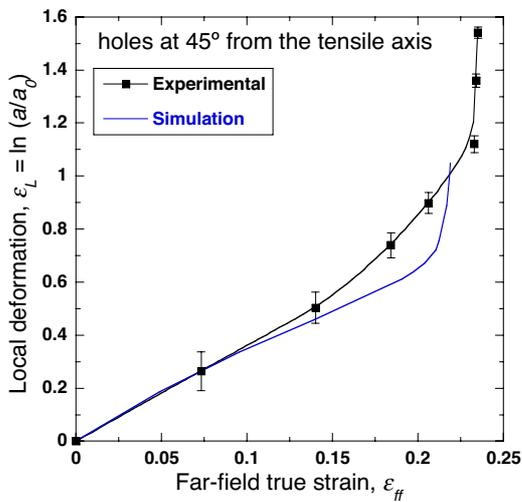
Figure 8: Experimental and numerical results of the evolution of the local deformation at the scale of the holes,  $\epsilon_L$ , as a function the far-field true strain,  $\epsilon_{ff}$ , for the sample with two holes orientated at  $45^\circ$  to the tensile axis and spaced  $37 \mu\text{m}$ .
