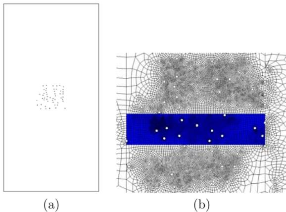
Figure 12: (a) Feature edges of the finite element model used to investigate void linkage in a random array of holes. (b) Detail of the finite element mesh in the hole region showing in dark the zone in which the nonlocal ductile damage model was included in the simulations.
