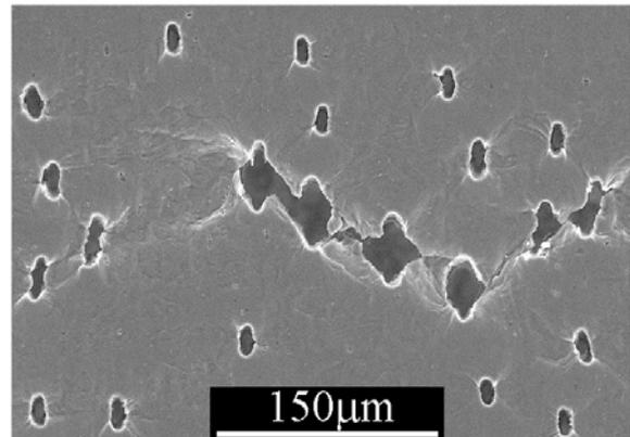
Figure 15: Micrograph of the fracture path after void linkage in the sample with a random array of holes.
