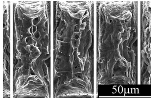
Figure 3: Fracture surface of a sample containing a regular array of holes oriented  $90^\circ$  with respect to the tensile axis. The sample fails by internal necking and the coalescence of secondary voids between the main laser drilled holes. The vertical white lines indicate the locations of the laser drilled holes.
