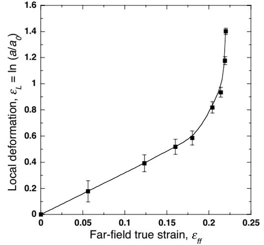
Figure 2: Experimental result showing the evolution of the local deformation at the scale of the holes,  $\varepsilon_L$ , as a function the far-field true strain,  $\varepsilon_{ff}$ , for the sample depicted in figure 1.
