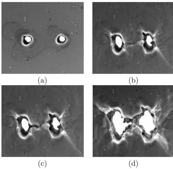
Figure 1: Scanning electron micrographs obtained *in situ* during the tensile deformation of the 5052 Al alloy sample with two holes oriented at  $90^\circ$  with respect to the tensile axis (vertical) and  $37 \mu\text{m}$  apart. The far-field true strain,  $\varepsilon_{ff}$ , for each micrograph was: (a) 0.0, (b) 0.204, (c) 0.213 and (d) 0.220. This last micrograph corresponds to the instant of void linkage as the intervoid ligament is broken.
