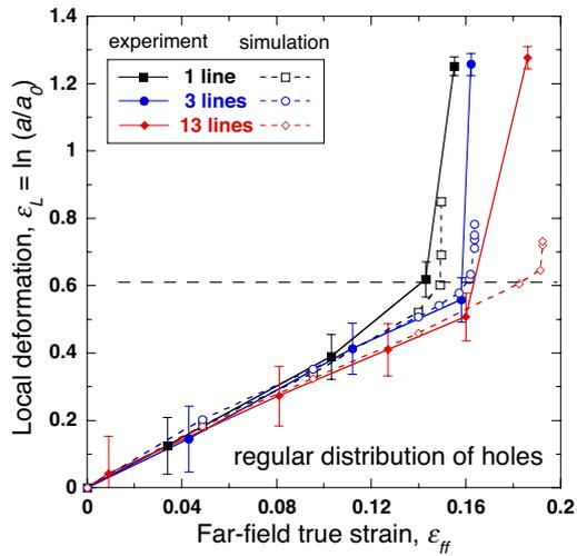
Figure 11: Numerical and experimental results on the evolution of the local deformation at the scale of the holes,  $\varepsilon_L$ , is plotted as a function the far-field true strain,  $\varepsilon_{ff}$  in samples with 1, 3, and 13 lines of holes along the tensile axis.
