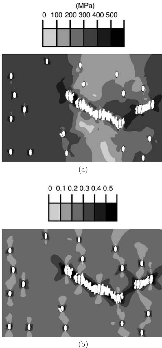
Figure 14: Numerical simulation of the fracture path after void linkage in the sample with a random array of holes. (a) Contour plot of the Von Mises equivalent stress. The white regions correspond to the elements which have been deleted from the finite element mesh due to damage. (b) *Idem* as (a) but the contour plot shows the accumulated plastic strain.
