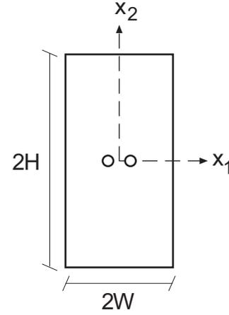
Figure 4: Schematic of the sample for the simulations for the model with two holes oriented at  $90^\circ$  with respect to the tensile axis and spaced  $37 \mu\text{m}$ . Drawing not to scale.
