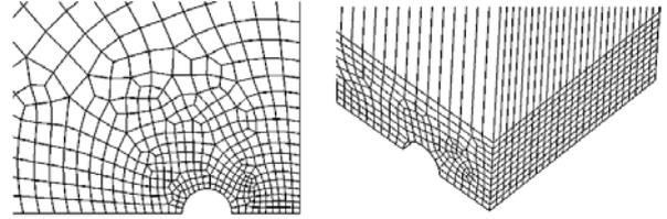
Figure 5: Details of the finite element discretization (in two and three dimensions) of the sample with 2 holes oriented at  $90^\circ$  with respect to the tensile axis.
