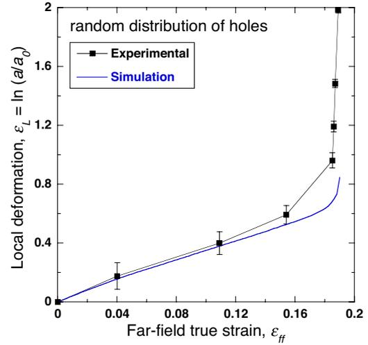
Figure 13: Numerical and experimental results on the evolution of the local deformation at the scale of the holes,  $\varepsilon_L$ , plotted as a function the far-field true strain,  $\varepsilon_{ff}$  in the sample with a random array of holes.
