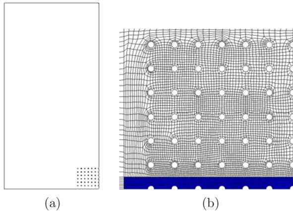
Figure 10: (a) Feature edges of the finite element model used to investigate the effect of regular arrays of holes on void linkage. (b) Detail of the finite element mesh in the hole region showing in dark the zone in which the nonlocal ductile damage model was included in the simulations.
